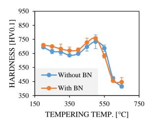
Left: Austenization chart. Right: Tempering hardness. BN: Boiling nitrogen as a cryogenic treatment.
